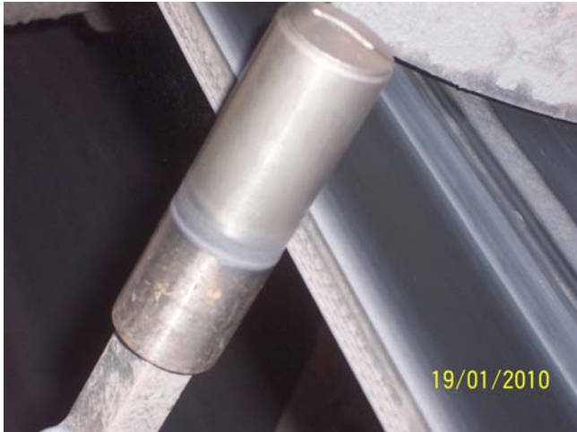
Photo 1 (Signs of wear on LHS tail drift switch.)
