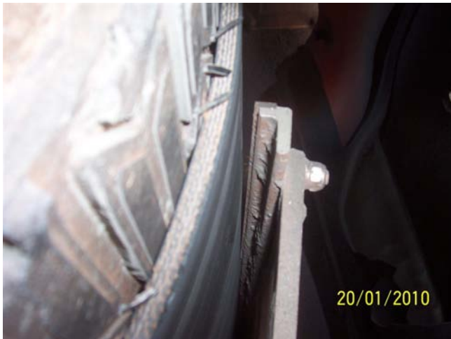
Photo 4 (Primary cleaner requires closer positioning to belt.)
