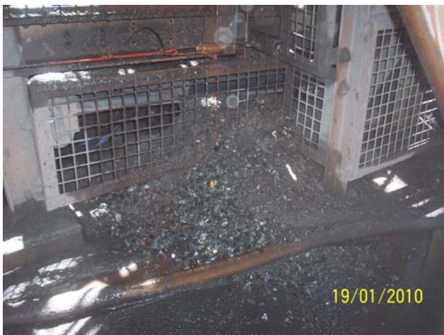
Photo 4 (Excess build-up around LHS/RHS of plough.)
