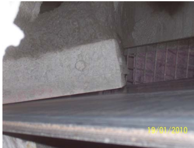
Photo 2 (Plough at tail build-up on blade and poor nose contact.)
